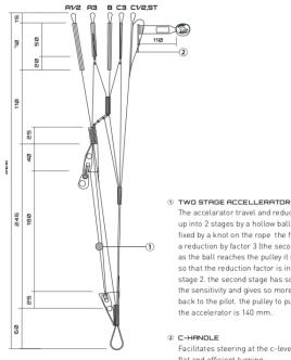
The accelarator travel and reduction is split up into 2 stages by a hollow ball its position is fixed by a knot on the rope the first stage has a reduction by factor 3 (the second stage by 2) as the ball reaches the pulley it is blocking it
